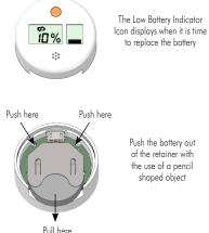
Push the battery out of the retainer with the use of a pencil shaped object
