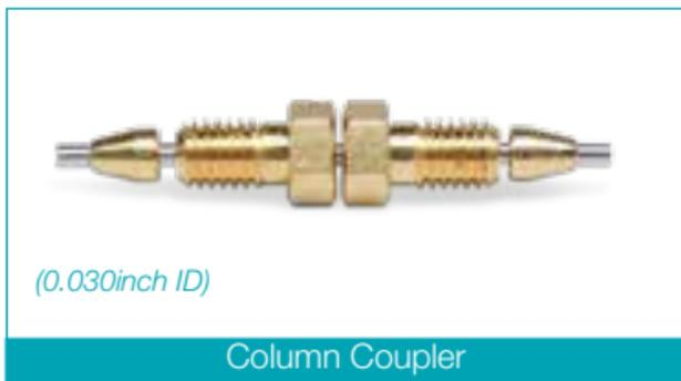
Proper seating of these fittings will eliminate voids or leaking. Hand tighten the fittings, then using a 1/4 inch wrench, tighten up to 1/4 turn more to ensure a leak-tight fitting.
