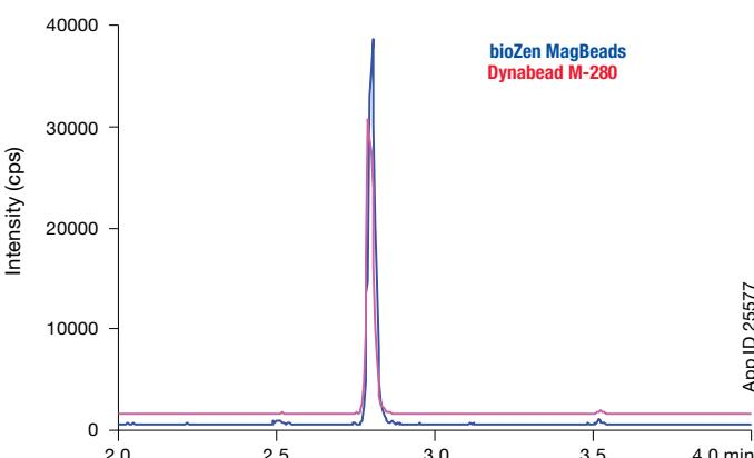
By switching to the bioZen 2.6 µm Peptide XB-C18 we were able to quantify 6 signature peptides from the digestion of Rituximab with excellent recovery and sensitivity for all peptides using only a 50 mm bioZen Peptide column. The chromatogram below displays the recoveries seen for a 1 µg injection of digested sample (**Figure 3**).
