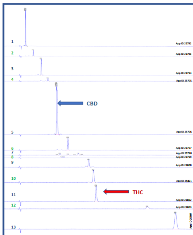
Chromatograms of collected fractions From CBD extract on 100 x 21.2mm, Axia prep column Flow Rate = 20 mL/min Injection Volume = 100 µL
