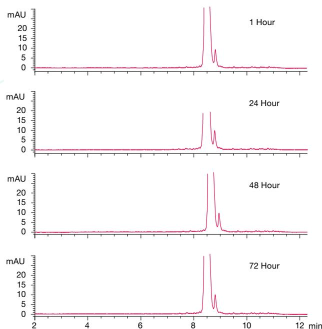
**50 µL Injected:** IEX column, DNAPac® PA200 250 x 4.0 mm
