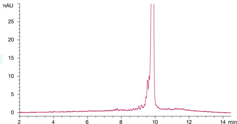
**50  $\mu$ L Injected:** IEX column, DNAPac<sup>®</sup> PA200 250 x 4.0 mm
