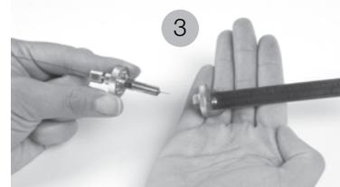
3. Unscrew the installation gauge and install the nut and column into the instrument.
