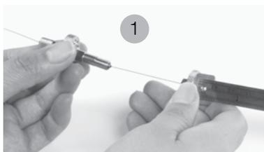
1. Insert column through column nut and ferrule. Cleanly cut  $\geq 1$  cm of the column that is protruding from the nut and ferrule. Insert the end of the column and column nut into the bottom of the Cool-Lock Nut Installation Gauge.
