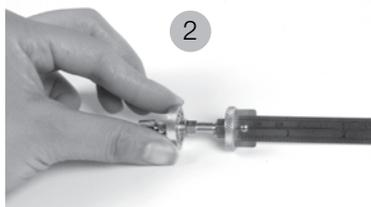
2. Hand-tighten the column nut into the gauge until the ferrule starts to compress. Adjust the length of the column to the desired length. Further tighten the nut into the gauge until the column cannot slide. If using the Cool-Lock Nut, tighten its bottom ferrule. Make sure lower body/ferrule is in the full extension position. Otherwise, mark the column at the base of the column nut to ensure the correct installation depth after installation.
