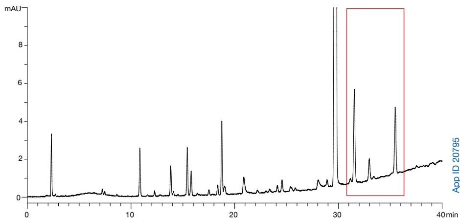
b. Phenomenex Kinetex® 5 µm C18 250 x 4.6mm; Backpressure = 188 Bar
