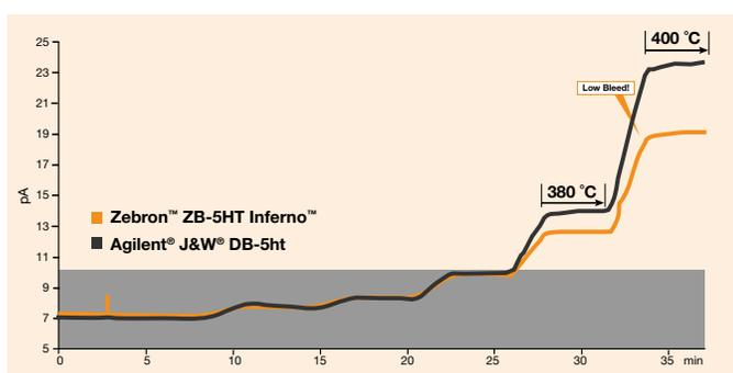
**Figure 2.** Bleed comparison of the DB-5ht and ZB-5HT Inferno. The shaded area depicts the bleed criteria for MS certified columns on a MS detector. MS bleed certification values are typically read at 320 °C. The ZB-5HT demonstrated lower bleed than the DB-5ht. It meets MS certification limits, even at 360 °C.
