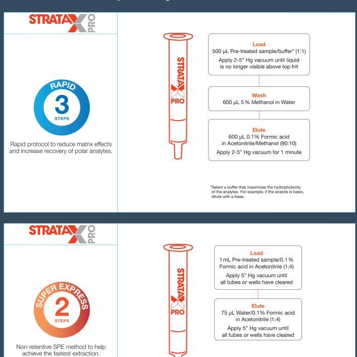
Protocols are written for 30 mg/1 mL tubes, adjust based on sorbent size.
