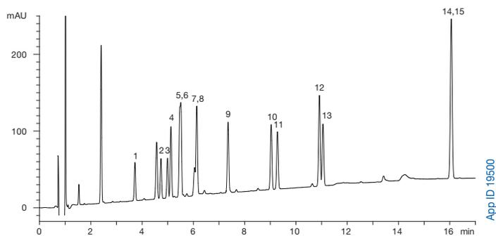
**Figure 1** illustrates the ability of the Kinetex XB-C18, 2.6 µm core-shell column to rapidly screen and separate all 15 compounds. In this separation, the Kinetex XB-C18 column offered the highest peak capacity of all of the five columns used in the experiment. Peak capacity is the best measure of performance for a gradient separation and high peak capacity values indicate increased analyte resolution over a given analysis time.
