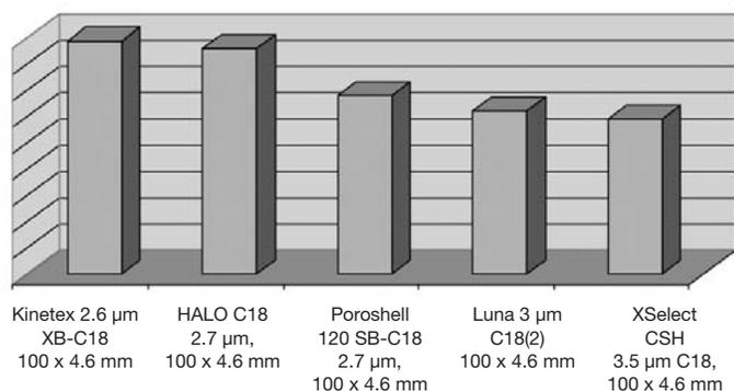
Based on the peak capacity data generated and represented in **Figure 6**, it is apparent that the three core-shell silica HPLC technologies provide an advantage over the two fully porous silica products used in the experiment when it comes to resolving power. **Figures 1-5** also indicate that the core-shell columns provide higher signal response due to the very narrow peak widths achieved, which allow for lower levels of detection for analytes present in lower concentration.
