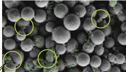
Scanning electron microscopy of column inlet frit
