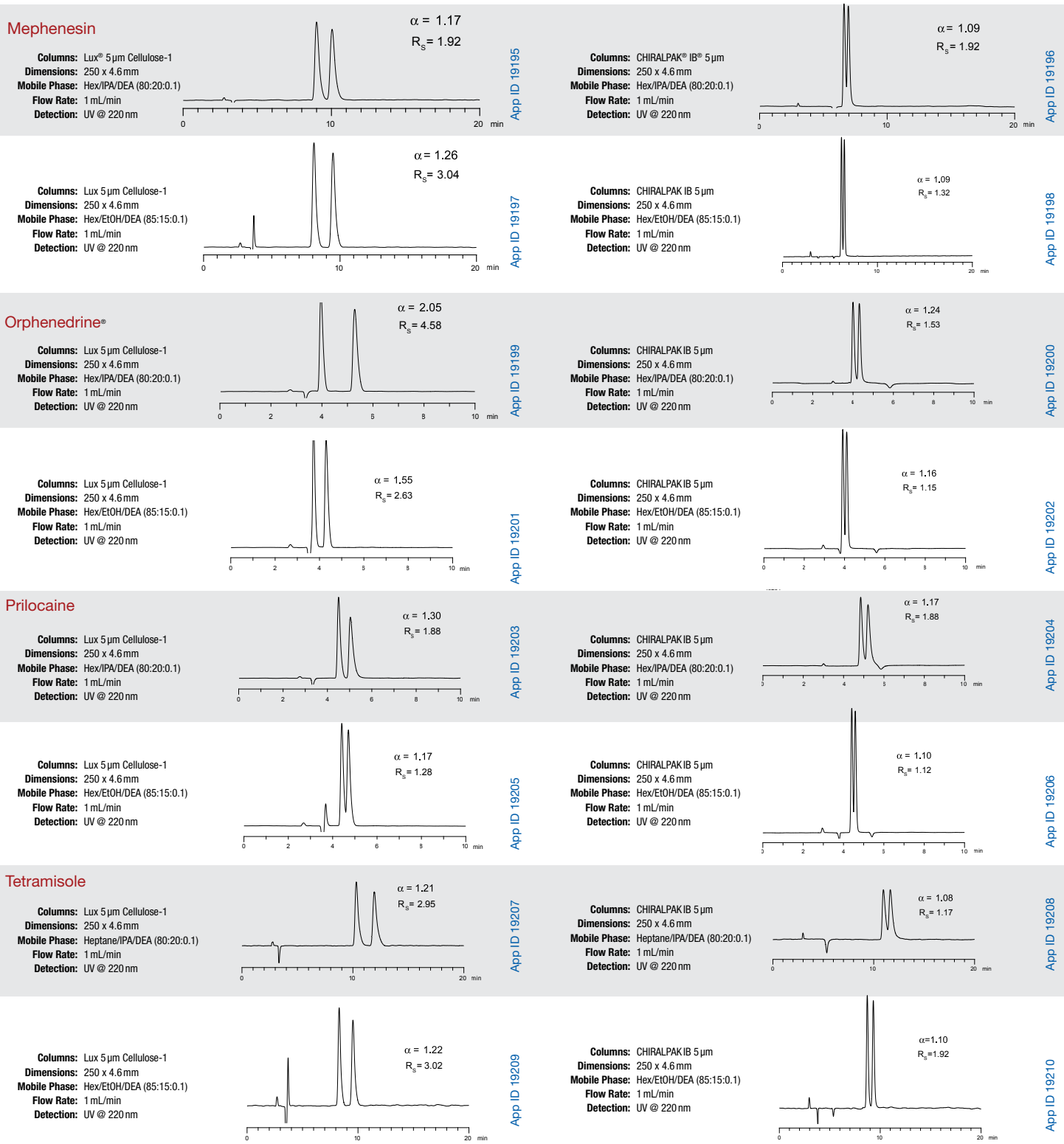
Figure 5. Effect of Organic Modifier on Lux Cellulose-1 (coated) and CHIRALPAK® IB® (immobilized) CSPs
