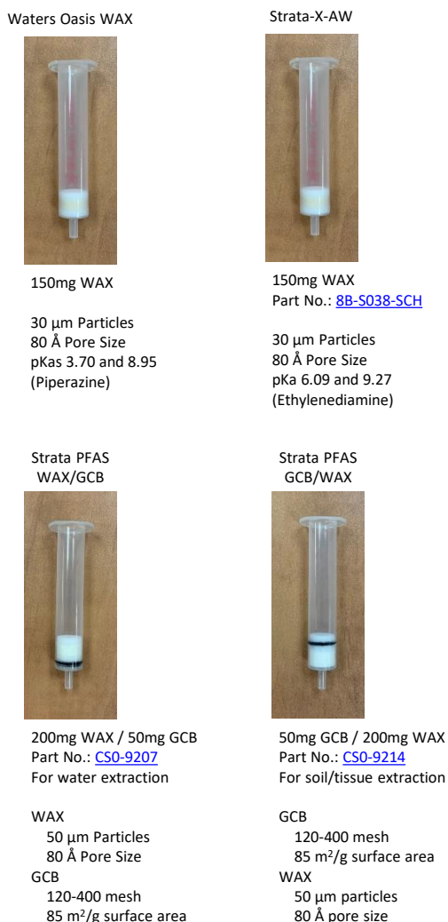
Figure 1. SPE Cartridges Used for the Comparison Study. Note the Order of the WAX/GCB vs. GCB/WAX for the Water and Soil Matrices, Respectively.
