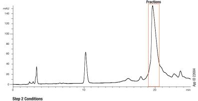
Conditions same as Step 1, except as noted: Mobile Phase: A: 0.1 % TFA in Water B: Acetonitrile Gradient: Time (min) % B 0 10 5 10 20 20 25 20 Sample: Bivalirudin Step 1 Product
