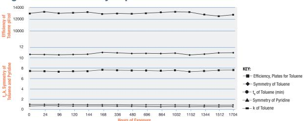
$Test \ Conditions: \ Column \ stability \ tested \ under \ highly \ basic \ conditions. \ Continuous \ flush \ in \ 20 \ mM \ Na_{2}HPO_{4} \ (pH \ 10.0) \ in \ Water/Acetonitrile, 50:50.$
