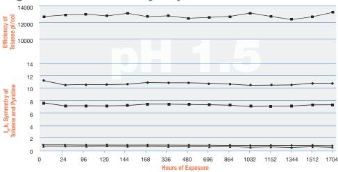
Test Conditions: Column stability tested under highly acidic conditions. Continuous flush in 0.1 % TFA (pH 1.5) in Water/Acetonitrile, 50:50.
