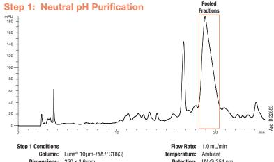
Dimensions: 250 x 4.6 mm Part No.: 00G-4616-E0 Mobile Phase: A: 20 mM Potassium phosphate pH 7.0 B: Acetonitrile Gradient:
