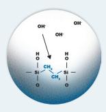
Multi-Point Ligand Attachment Resists Low pH Ligand Cleavage
