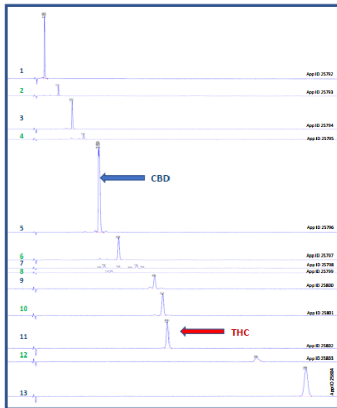
Figure 5 Chromatograms of collected fractions From CBD extract on 100 x 21.2mm, Axia prep column Flow Rate = 20 mL/min Injection Volume = 100 \mu L
