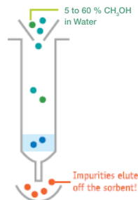
4. WASH IMPURITIES with 1 mL 5-60 % Methanol in D.I. Water and dry for 30 sec. at full vacuum
