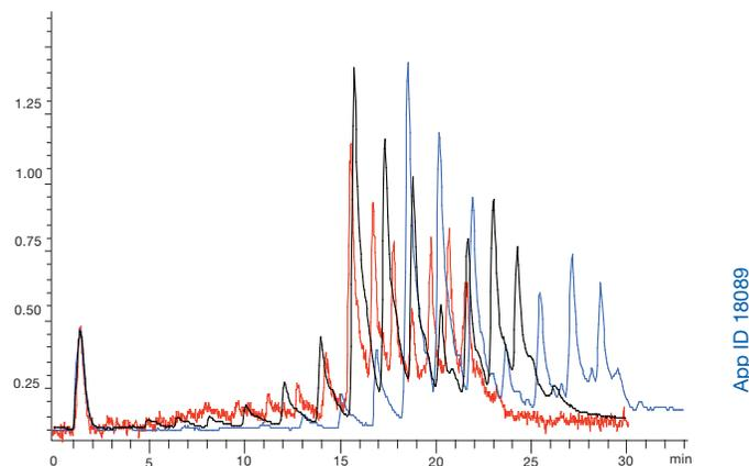
Different ratios of HFIP to TEA were investigated using the poly dT 12-18 standard mixture. HFIP was fixed at 200 mM and different levels of TEA were used between 1 and 20 mM (4 mM-Red trace {pH 7.6}, 8 mM-Blue trace {pH 8.0} and 14 mM-Black trace {pH 8.3}). Optimal retention, MS response, and resolution were observed for the 200 mM HFIP/ 8 mM TEA mobile phase mixture.
