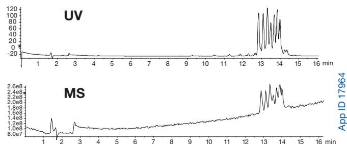
LC/MS TIC and UV-Vis Chromatogram from the same run shown together of a poly dT standard run on a Clarity® Oligo-RP™ column. Note the reduced resolution from the MS chromatogram. MS sampling rate and post column void volume can dramatically affect the efficiency and resolution of closely eluting oligonucleotide peaks.
