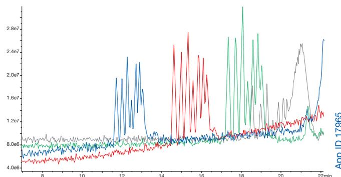
LC/MS separations of a 12-18 dT oligonucleotide standard using different ion-pairing concentrations. Concentrations used were: Black trace) 15 mM TEA/ 400 mM HFIP, Green trace) 2.8 mM TEA/ 280 mM HFIP, Red trace) 4 mM TEA/ 100 mM HFIP, Blue trace) 2 mM TEA/ 50 mM HFIP. Note the increasing MS signal with reduced ion-pairing buffer concentration.
